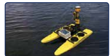
HyDrone™ ASV with Trimble SPS 585 and TSC3
