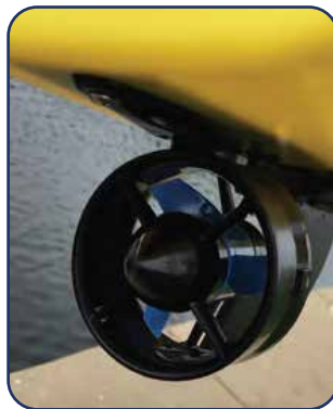
Power differential thrusters for maneuverability
