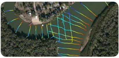
Bathymetric image using single beam echosounder.
