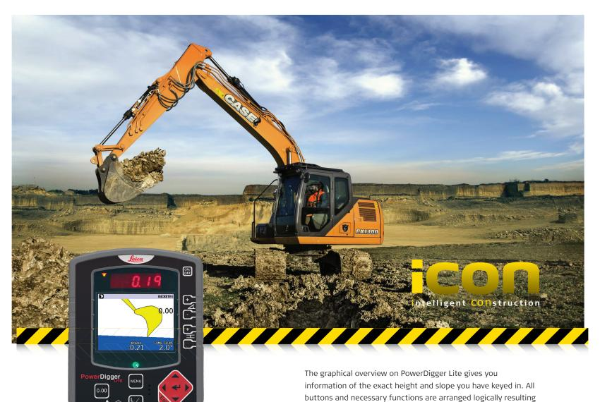
Leica PowerDigger Lite is a simple, economical excavator control solution, ideal for contractors who want to enter into machine control. The single slope control box with multicolour display is easy-to-use, user definable and can be upgraded easily to a 2D dual slope system as needed.
