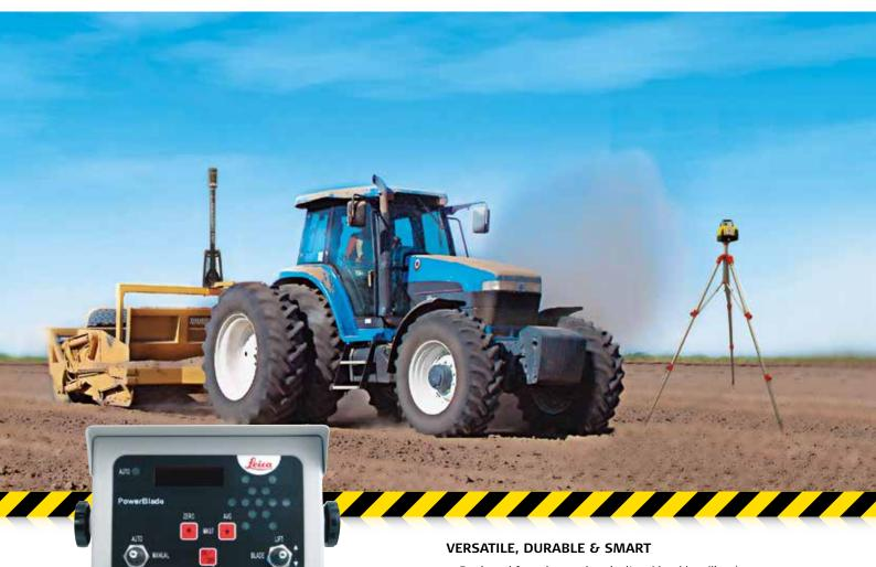
The Leica PowerBlade system is a complete solution steered by the MCP700 control box – easy-to-use and full of features. A choice of laser receivers allows you to tailor the system to your application. An extremely rugged electric mast and a variety of hydraulic options complete the system.
