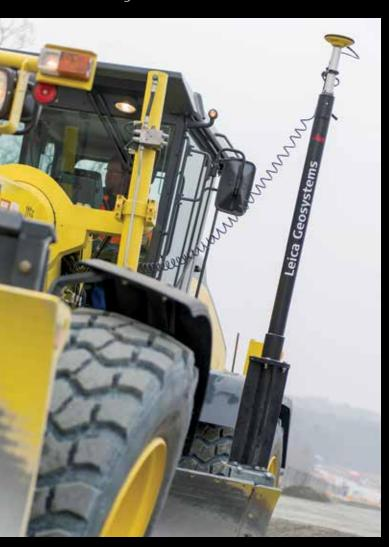
The iCON iGG4 enables motor grader operators to do more without spending years in on-the-job training. The easy-to-understand solution makes most operators productive in just a short period of time – crab walk when creating ditches or grading side slopes – operators won't have to watch both ends of the blade because iGG4 does it for them. The bottom line is: save money by getting more production out of the machines you already own by adding an iCON grade iGG4 to your grader.
