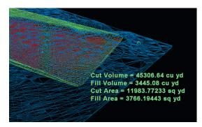
Ground surface TINs and other meshes are easily created and offer great value. Here is an automated report analyzing cut and fill quantities using before-and-after scan data of a ground surface.
